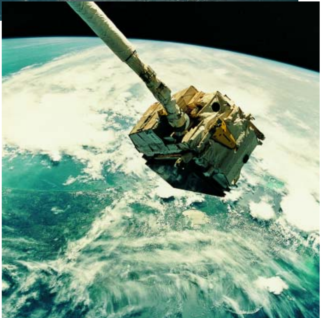
Eureca – with its solar wings already folded against its sides – was recaptured in June 1993 after almost a year in orbit. (NASA)
